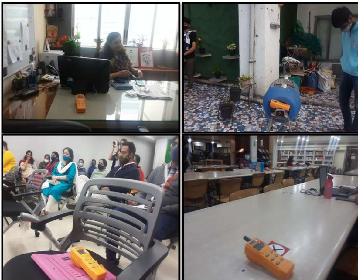
CO 2 level measurement at various locations of UPG College
